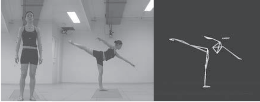
Figure 5.9 From left to right: dancer with retro-reflective markers according to the PlugInGait marker set from VICON; still from a conventional video sequence; and the corresponding stick figure obtained from the 3D analysis.
