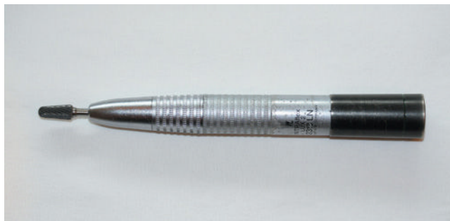
Figure 16.56 Acrylic trimming bur in straight handpiece.
