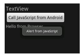
Figure 7.4: Communicating between Android and an embedded Web-View
