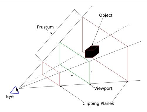
Figure 10.1: Viewing a three-dimensional scene
