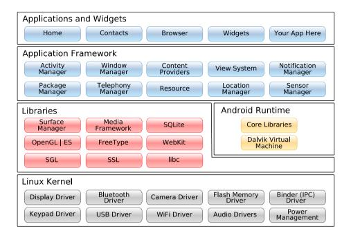
Figure 2.1: Android system architecture
