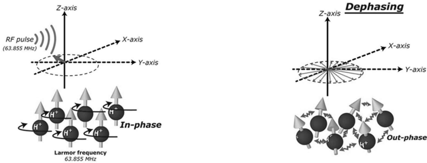
FIGURE 2.4 Alignment of protons in in-phase and out-phase conditions.
