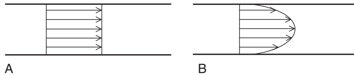
FIG. 2.21 The velocity profile for blood flowing through an artery that is modeled as an inviscid fluid (A) or a viscous fluid (B). An inviscid fluid has a uniform velocity profile because there is no internal resistance to motion. A viscous fluid has a nonuniform velocity profile, which can be idealized to a parabolic velocity profile for many conditions.
