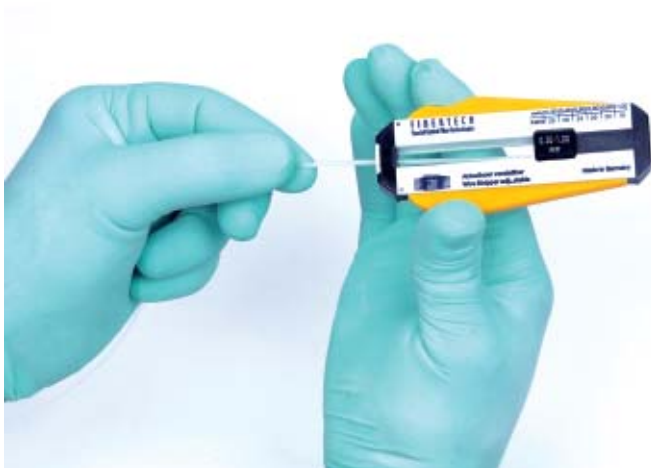
Fig. 10.8B: Stripping of the laser cable
