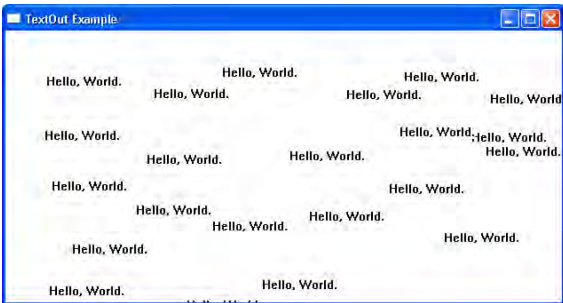
Figure 15.2: We output the text "Hello, World." wherever the user presses the left mouse button.
