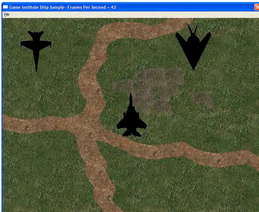
Figure 17.10: The backbuffer after the mask bitmap is drawn to it. It marks the pixels black where we will copy the image bitmap to.
