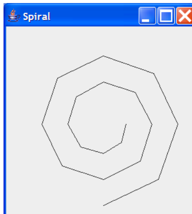
Fig. 12.33 | Spiral drawn using method drawPolyline .
