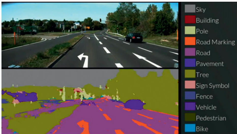
Figure 8.1 Machine learning technology behind self-driving car. (Source: YouTube: Deep Learning: Technology behind self-driving car. 5 )
