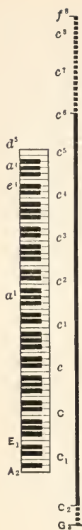
FIG. 13. The Series of Auditory Qualities. The keyboard of a grand piano extends from the A_2 of 27.5 vs. to the c^8 of 4224 vs. The smaller piano keyboard ranges between the C_1 of 33 vs. and the a^4 of 3520 vs.
