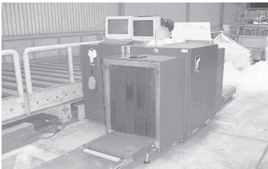
Figure 2 Type of X-ray Technology Used by Some Foreign Air Carriers to Inspect Air Cargo Bound for the United States
