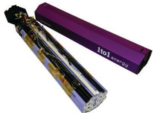
Figure 15.3 E-bike battery pack: a Stromer power battery.
