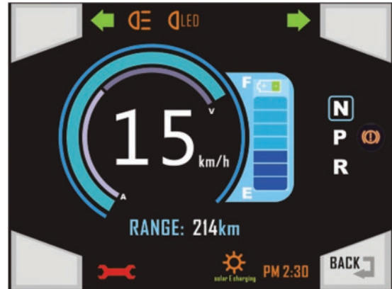
Figure 14.4 Electric vehicle instrument displaying all kinds of information.
