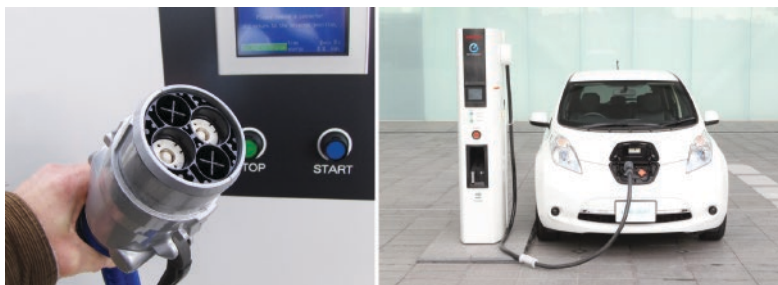
Figure 10.6 CHAdeMO connector. Credit: C-CarTom / Wikimedia Commons / CC BY-SA 3.0 and Nissan CHAdeMO level-3 Charger. Credit: Caxton & CTP Printers and Publishers Ltd.
