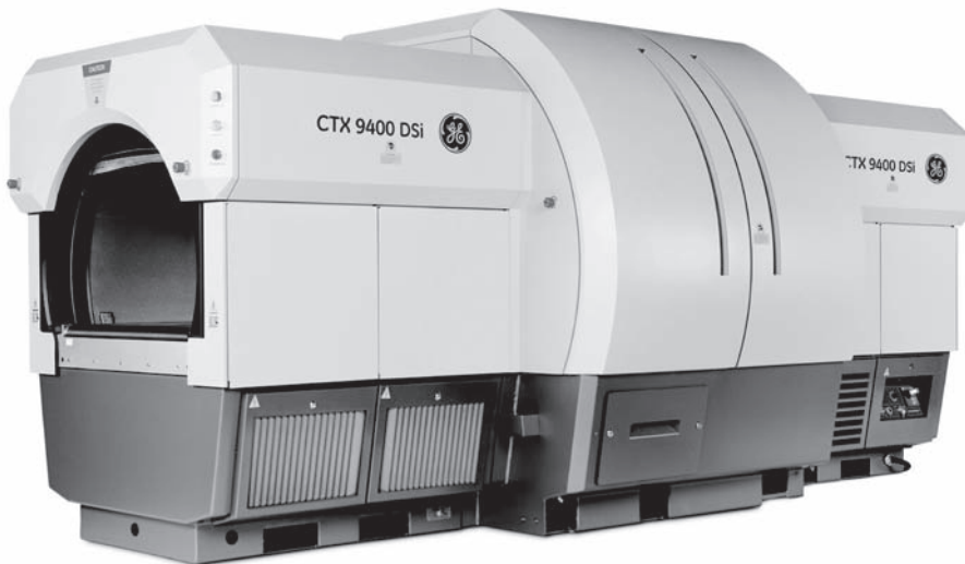
FIGURE 9.4 The CTX 9400 is GE Security's most sophisticated inline explosive detection System (EDS) and the second EDS in its Multi-Generational Product Plan for such systems. The system utilizes core technology derived from medical computed tomography. The projection x-ray images initially created determine which bags or cargo need slice images taken by a rotating x-ray source which can then be further analyzed and compared with the properties of explosives. (Image courtesy of GE Security)
