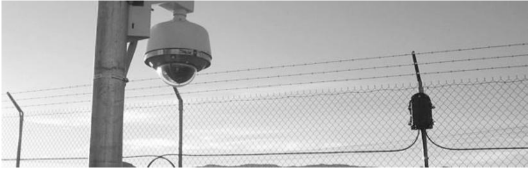
FIGURE 15.1 The FiberPatrol® FP 1100 series features fiberoptic sensor technology available for fence-line perimeter security. These location-sensing intrusion detection systems are distinguished by their ability to pinpoint the absolute location of an intrusion attempt to within one or two fence panels. (Photo courtesy of Optellios, Inc.)
