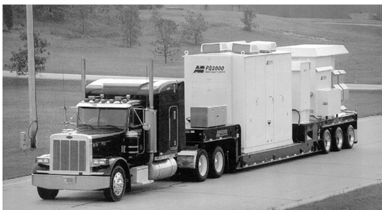
Fig. 9.4 AC Battery PQ2000 system on a truck slated for delivery. The PQ2000 is the forerunner of the current S&C Electric Company PureWave ® system
