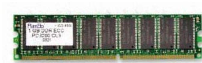
The advantage of RAM is that, due to its architecture, the transfer speeds are infinitely faster than that of a hard drive. On the downside, it is also infinitely more expensive per GigaByte, and because the data is stored by means of electrical charges, information cannot be stored *or maintained* unless your computer is running.
