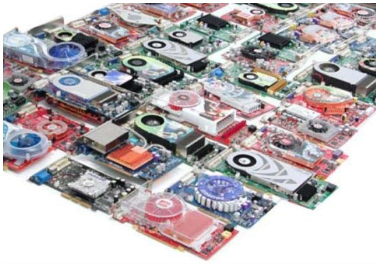
The graphics card is an expansion card with a GPU (graphical processing unit) chipset, dedicated to graphics rendering. Their main purpose is to render, and output (3D) images to a monitor. Though most motherboards (more about them later on in the guide) have built-in GPU chips, they are normally not sufficient for gaming. Rather, we'd like to use an external component that can be switched and upgraded without need to buy a whole new computer.
