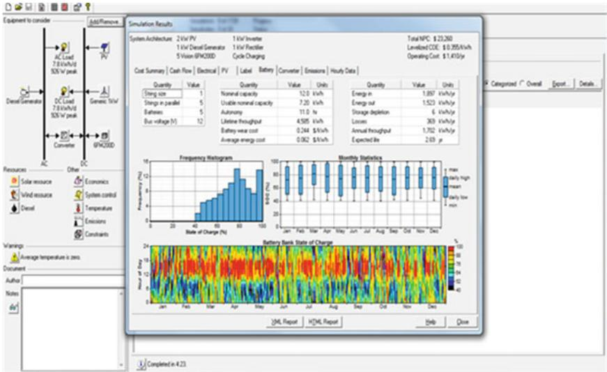
Fig. 5.15 Battery electrical performance
