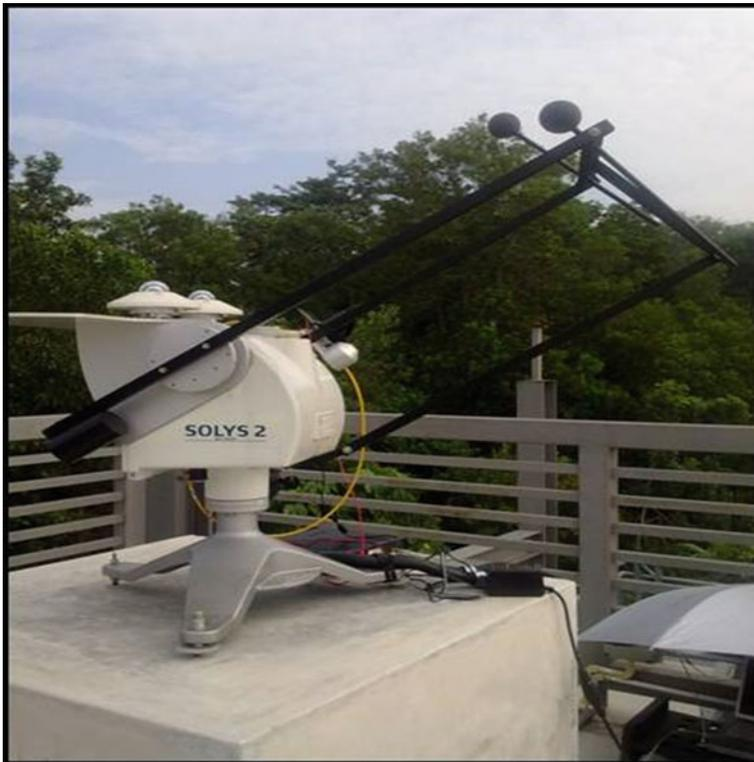
Fig. 2.2 Sun tracking system equipped with solarimeter
