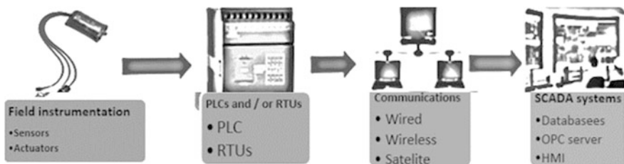
Fig. 5.1 Conceptual illustration of ICS/SCADA infrastructure developed
