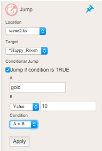
Figure 5-4. The Jump component window in TyranoBuilder in conditional mode
