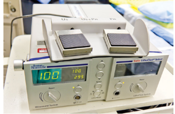
Figure 8.5 Swiss LithoClast Select. As printed on the foot pedal, the surgeon has the ability to selectively activate both the ultrasound (Us) and pneumatic (Pn) modalities.
