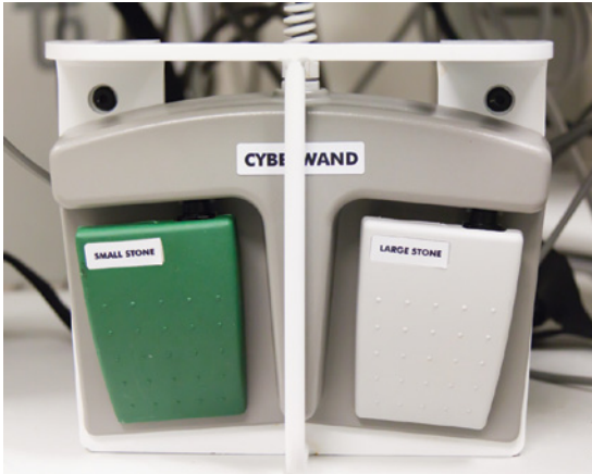
Figure 8.4 The CyberWand's foot pedal system. The pedal on the left activates only the inner ultrasonic probe (small stone). The pedal on the right activates both the inner and outer probes (large stone).
