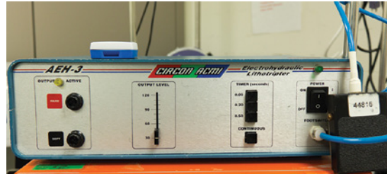
Figure 8.7 Example of an EHL lithotripter, the Circon ACMI AEH-3 with foot pedal.
