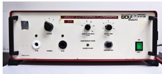
Figure 8.8 Another example of an EHL lithotripter, the Wolf 2137.50.
