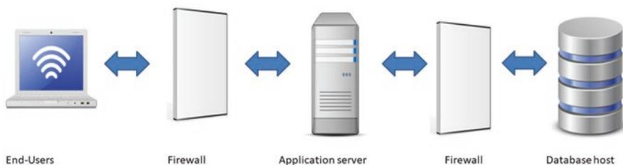
Fig. 6.9 Defense-in-depth mechanism
