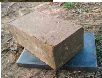
The CEB press (left), nicknamed "The Liberator," turns local soil into energy-efficient compressed earth blocks (below).
