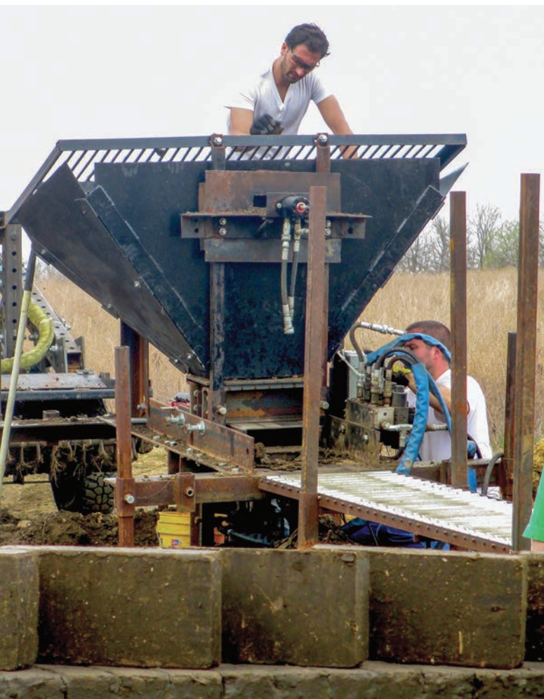
The CEB press (left), nicknamed "The Liberator," turns local soil into energy-efficient compressed earth blocks (below).
