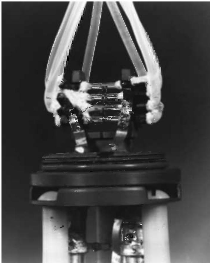
**FIGURE 8.2** Picture of the first four-coil flow-through multiplex-sample NMR probehead. A description is found in the text. (Reprinted from MacNamara et al. [8]. With permission from Elsevier.)
