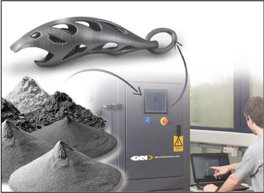
Fig. 2 GKN powder metallurgy—a bottle opener as an example of additive manufacturing (GKN 2017)
