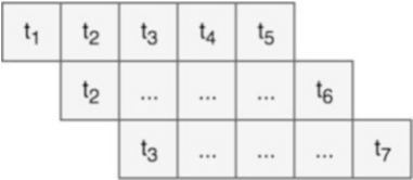
Fig. 4 Every second an audio slice is recorded; these slices are joined to give a single sequence that can be interpreted by the neural network
