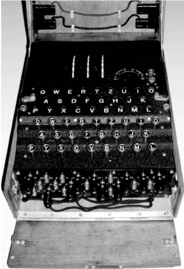
Figure 2.5. The Enigma cipher (Courtesy of T.B. Perera and the Enigma Museum).
