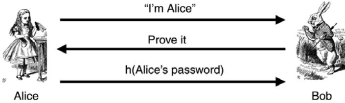
Figure 9.5. Simple authentication with a hash.
