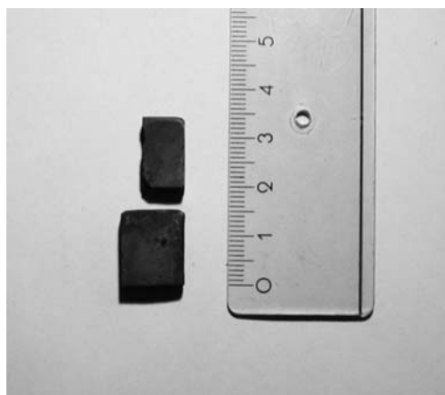
Figure 6.10 Bulk nanocrystalline nickel-free stainless steels samples.
