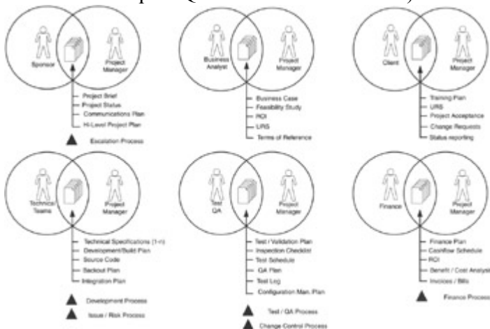
Figure 7.1: Project templates per project role.
