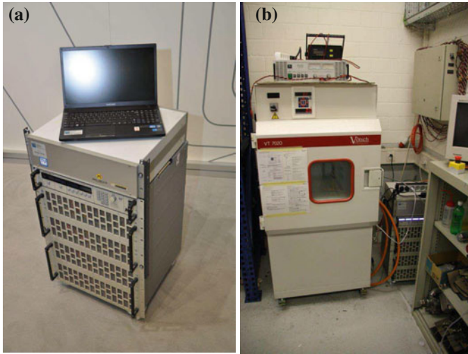
Fig. 3.1 Battery cell tester ( left ) and climate chamber ( right ) used to test different cell chemistries and temperatures
