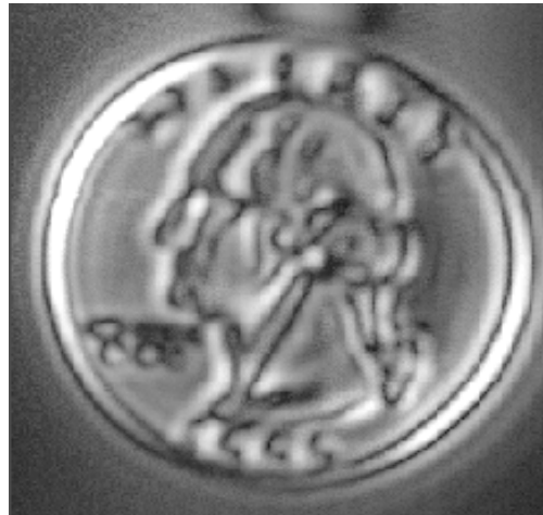
Fig. 2. Vibro-acoustic image of US quarter obtained with the setup of Fig. 1.
