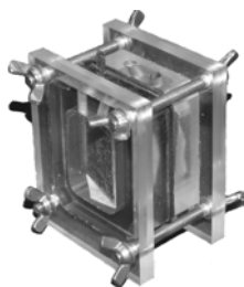
Fig. 2. Microbial Fuel Cell in its analytical form
