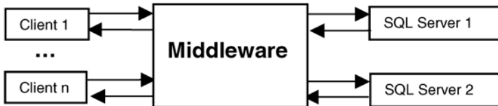
Fig. 1. Fault-tolerant server node (FT-node) with two or more diverse SQL servers (in this case two: SQL Server 1 and SQL Server 2 ). The middleware “hides” the servers from the clients ( 1 to n ) for which the data storage appears as a single SQL server.
