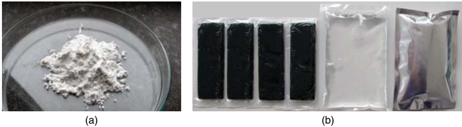
Figure 3.8 Picture of a microencapsulation of PCMs (courtesy of Rubitherm GmbH).
