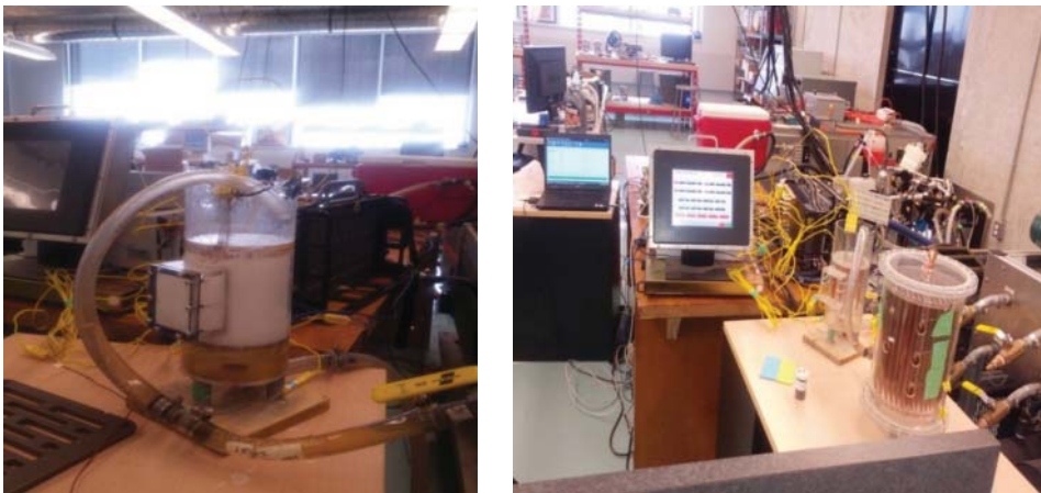
Figure 4.13 Solid phase of the PCM in the heat exchanger and test set up.
