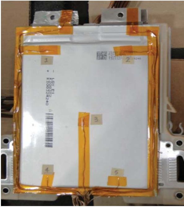
Figure 4.62 Location of thermocouples on the surface of Li-ion cells.
