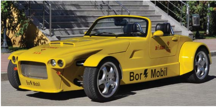
Figure 1.7 Sodium borohydride fuel cell vehicle (courtesy of TUBITAK Marmara Research Center).
