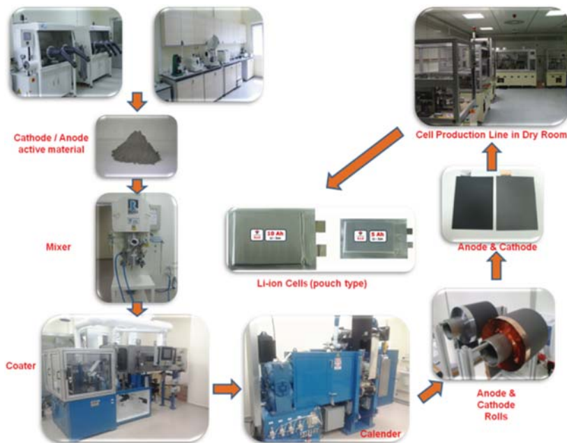
Figure 2.20 Conventional cell production methodology for Li-ion pouch cells (courtesy of TUBITAK Marmara Research Center).
