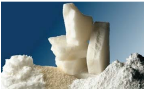
Figure 3.6 Picture of an organic PCM (courtesy of Rubitherm GmbH).
