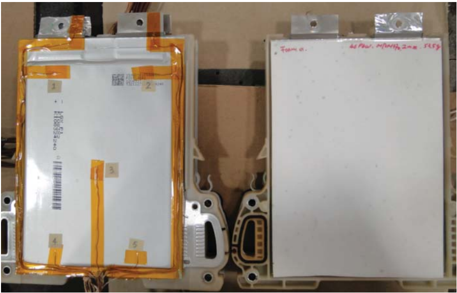
Figure 4.6 Connecting thermocouples on the surface of the Li-Ion cells.
