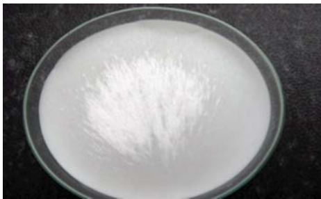
Figure 3.7 Picture of an inorganic PCM (courtesy of Rubitherm GmbH).
