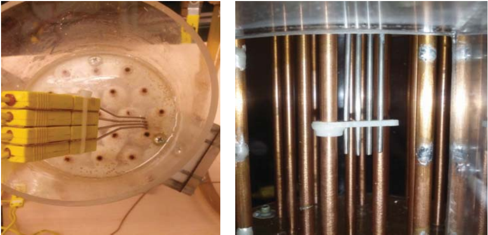
Figure 4.10 Position of thermocouples in equal distances from the copper tube.
