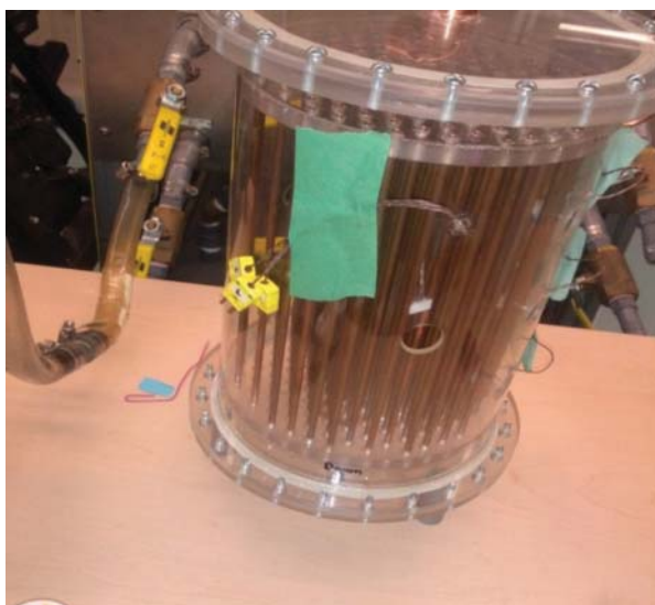
Figure 4.12 Manufactured heat exchanger with optimized dimensions.
