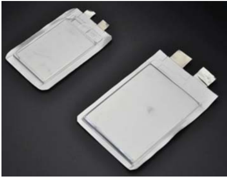
Figure 2.4 Sample pouch type lithium-ion battery (courtesy of TUBITAK Marmara Research Center).
