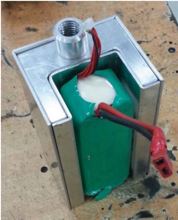
Figure 7.52 dry fit set up of the battery and the PCM jacket (Zafar, 2015).
