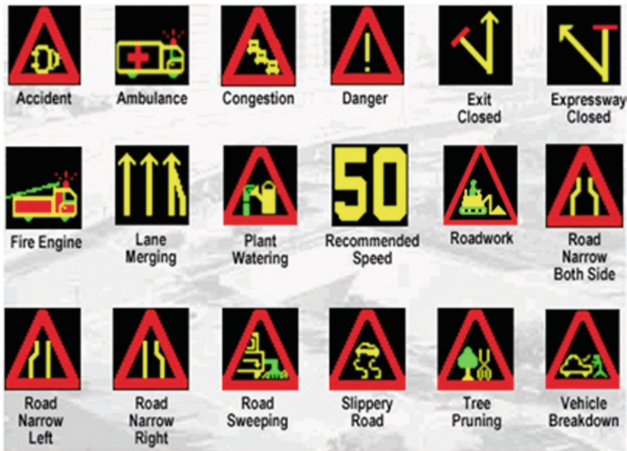
Fig. 18.4 Sub-optimal usability of EMAS displays arising from a design that is neither user nor task centric
