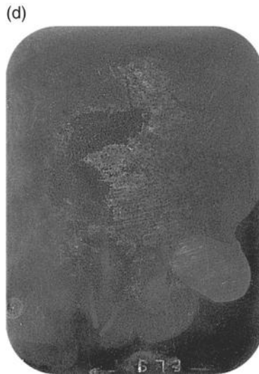
Figure 14.16 Radiograph handling faults: (a) scratched; (b) splashed; (c) crazed; (d) insufficient washing.
