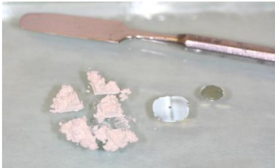
Figure 8.20 Zinc polycarboxylate cement – to mix.
