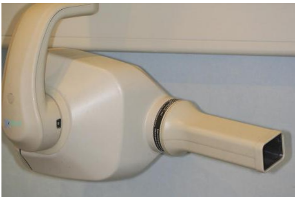
Figure 14.3 X-ray machine rectangular collimator tube.
