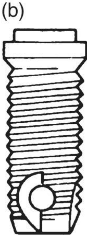
Figure 15.76 Dental implant components: (a) ball abutment for overdenture; (b) implant fixture.
