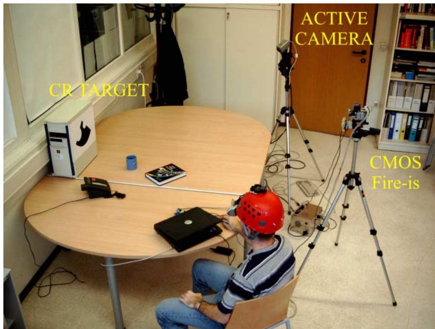
Fig. 11. This figure shows a setup for the verification of our approach. The cameras are mounted on a tripod to eliminate a possible influence of the movements of the user who wears the AR helmet and places the 3D marker next to various objects on the table (error in depth ( t_z ) < 10 % for a trained user, if t_z < 4 m)
