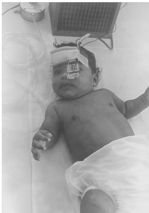
Figure 17.2 An eye-blink conditioning device for infants between 0 and 4 months of age (DeLucia, 1968). A stainless steel wire frame with a pair of Amperex germanium photocells mounted on two 16.76-mm pieces of Plexiglas. One photocell is focused on the sclera, and the other is focused on the lower lid. When the eye is open, ambient light reflects equally from both surfaces, producing no current flow. A blink reduces the light reflected from the sclera, producing a current flow proportional to the difference in light intensity on the two photocells. The output is fed into a polygraph adjusted to produce a full pen deflection when the eye is open. Secured in and projecting through the Plexiglas is a 7.94-mm (diam) nozzle through which a 2.5-psi air puff is delivered to the left corner of the infant's left eye from a distance of 2.54 cm. The device is taped to the infant's forehead, leaving the eyelid unrestricted and unencumbered.
