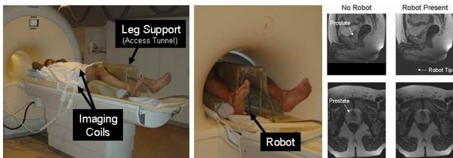
Fig. 5. Qualitative analysis of prostate image quality. Patient is placed on the leg support (left) and the robot sits inside of the support tunnel inside the scanner bore (center). T2 weighted sagittal and transverse images of the prostate taken when no robot components were present and when the robot was active in the scanner (right).
