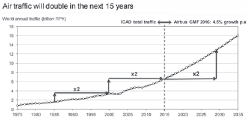
Figure 2.1 World Air Traffic 1974 to 2034. Traffic is measured in trillions of revenue passenger kilometers (RPK). One RPK represents one passenger flying one kilometer in air transportation. In the U.S., the more common statistic is the revenue passenger mile (RPM). Figure courtesy of Airbus, 2015.
