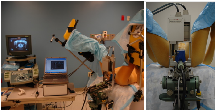
Fig. 2. System setup in the OR (left) and a closer view of the robot from the physician's perspective (right). Observe how the standard clinical hardware and setup are fully preserved.
