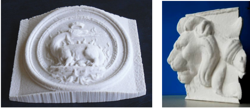
Fig. 4. Two replicas printed with resinated chalk. The undulate edges are due to an automated elaboration (exception made for the scale of the model, the selection of the printable area, and the thickening of the reconstructed surface). To obtain sharp edges a manual editing is needed.
