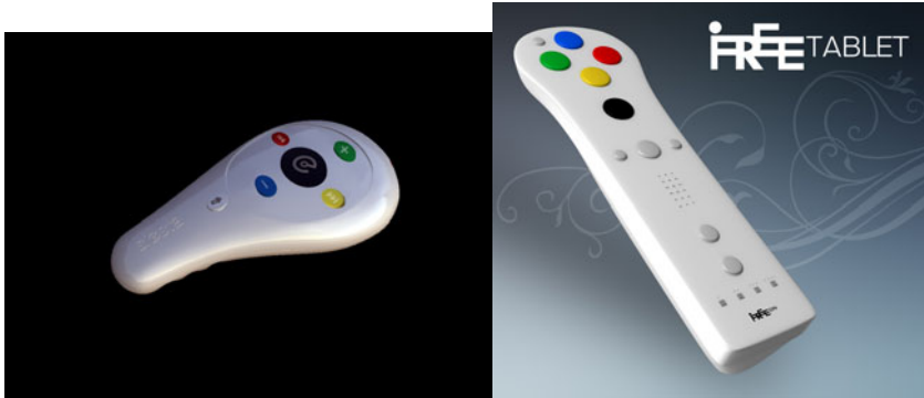
Fig. 3. Two iFreeMando models adapted with accelerometer and gyroscope
