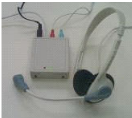
Fig. 6. Mouse system emulator with voice recognition
