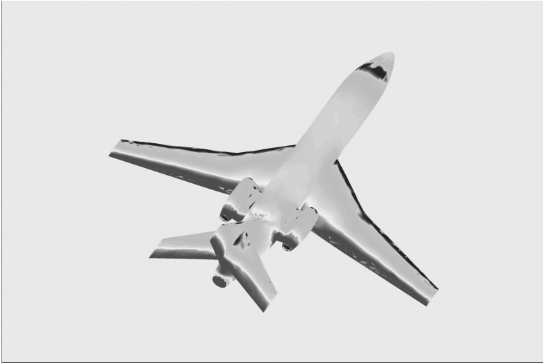
Fig. 2.1. Pressure color map from a RANS calculation [6] on a business jet performed in 1998 on a workstation (computed by Bijan Mohammadi).
