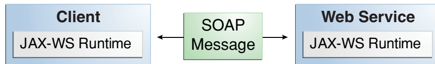
FIGURE 12–1 Communication between a JAX-WS Web Service and a Client
