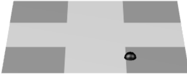
Fig. 2. This image shows the important part of the screen during the experiment. Three of the four grey squares are of base stiffness and a randomly selected one is stiffer. The white cross is softer and removes direction comparison between patches. The small sphere is the graphical representation of the haptic probe.
