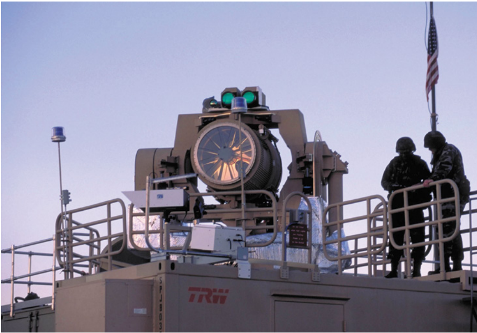
Figure 12.2 The Tactical High-Energy Laser, the world's first complete laser weapon. Source: The photo is by the US Army, and was released by them into the public domain.
