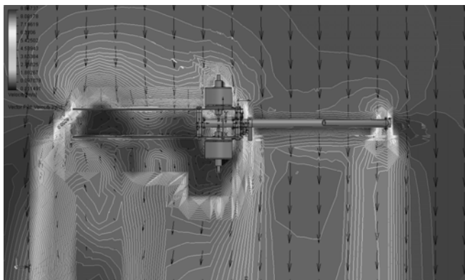
Fig. 5. Airflow simulation in SolidWorks. Light areas illustrate reduced air speed.
