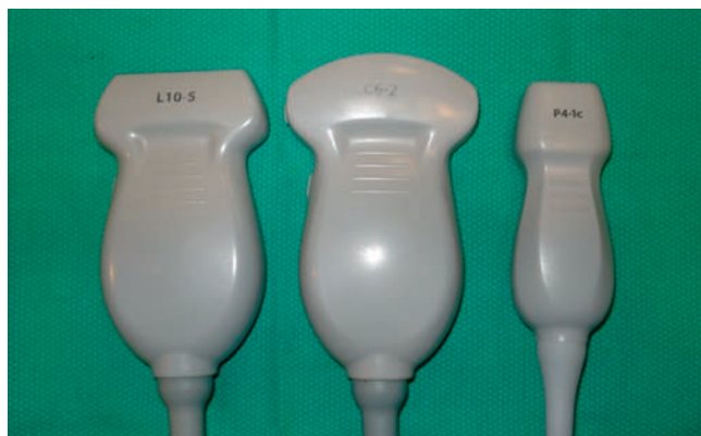
Figure 45-1. The three most commonly used probes. On the left is the high-frequency linear probe. In the center is a low-frequency curvilinear probe and to the right is a phased array probe.
