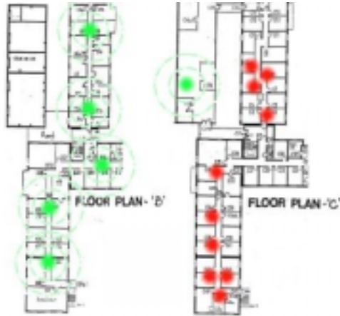
Fig. 7. Location of Hermes displays on 802.11b access points
