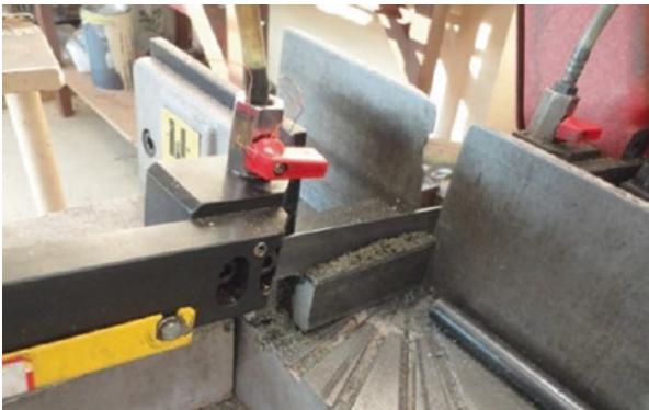
Fig. 25.1 Cutting of experimental samples on band saw
