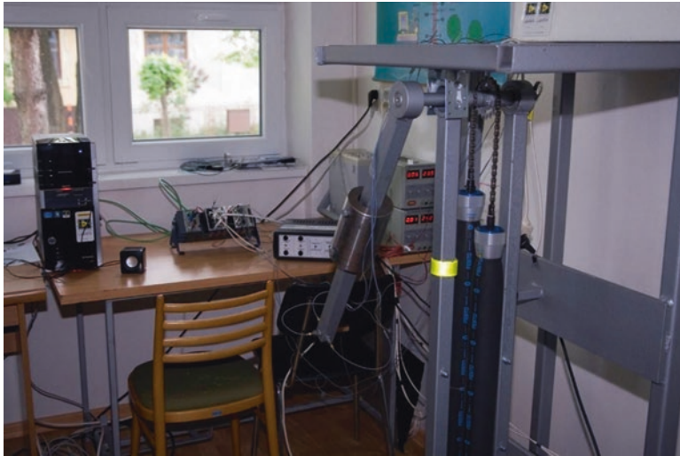
Fig. 4.3 Experimental device with drive based on PAM [7]
