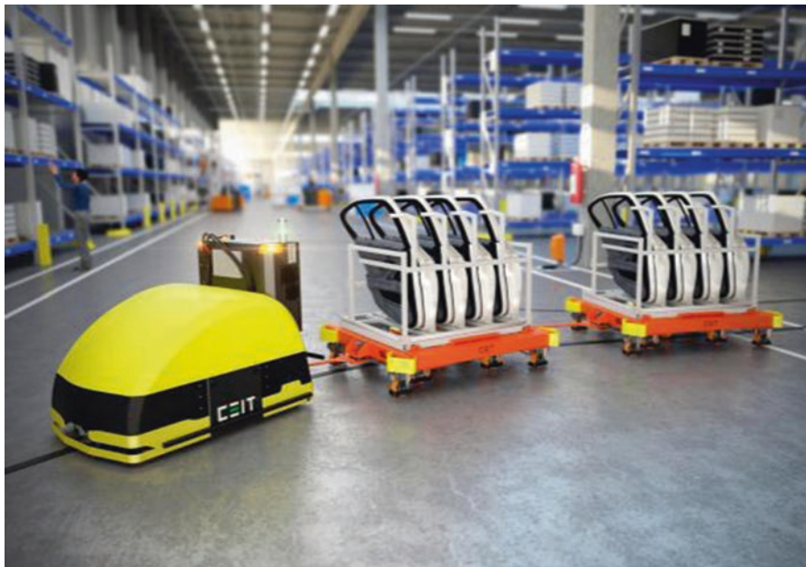
Fig. 13.13 CEIT AGV systems – towing version
