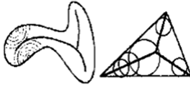
Figure 5.16. The figure on the left shows the skeleton of an object obtained by generating waves/fires from the boundaries of an object. The figure on the right shows the skeleton of an object obtained by using the maximum disk method.
