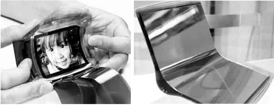
Figure 9.3 (top left) A flexible OLED TFT display; Figure 9.4 (top right) Sony VAIO concept with OLED/Bioplastic technology (Credits: SONY)
