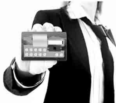
Figure 9.5 SmartDisplayer’s smart-card with e-paper display, combining OTP/RFID capability (Credit: SmartDisplayer.com)
