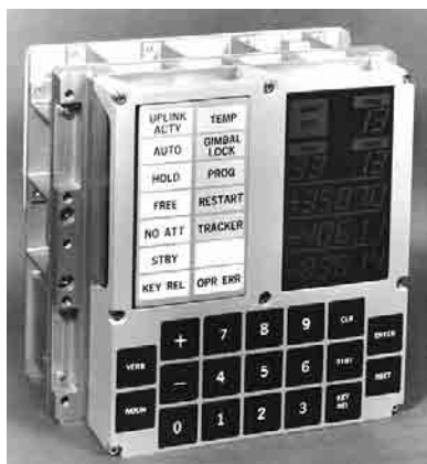
Figure 9.2 The Apollo Guidance Computer, circa 1970 (Credit: ComputerHistory.org)
