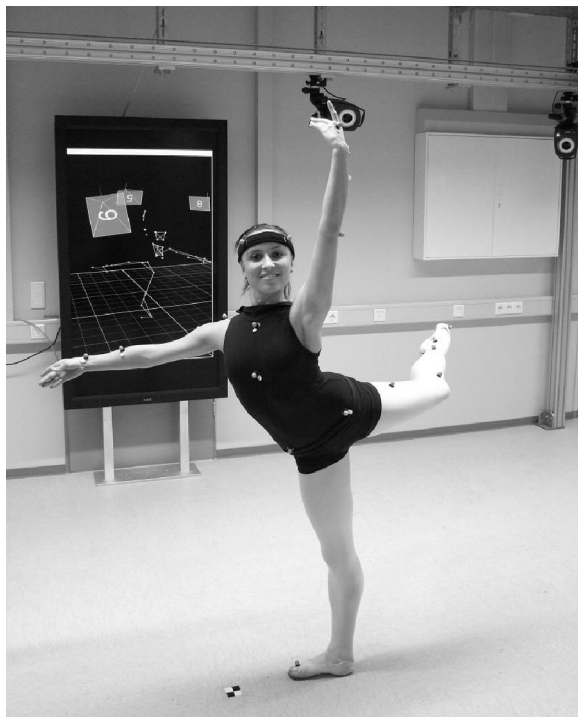
Figure 4.6 Dancer in the biomechanics lab. This dancer who is participating in a biomechanical study is equipped with retro-reflective markers on defined parts of her body. As she moves, 12 infra-red cameras (two of which are visible in the upper part of the picture) track the movement of these markers. The data collected by all cameras is sent to and integrated by a computer that calculates from this data a 3D model of the dancer's body (displayed on the monitor in the background) in real time. Dancer: Tanja Rastvorov. Photographer: Stefan Krüger, Research Institute for Cognition and Robotics (CoR-Lab), Bielefeld University.
